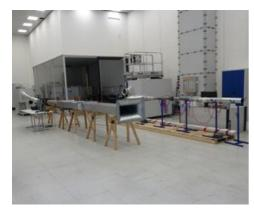
Test facilities in accordance with EN 12589: control tolerance; control response; pressure loss; characteristics for various upstream conditions; master-slave, etc.
